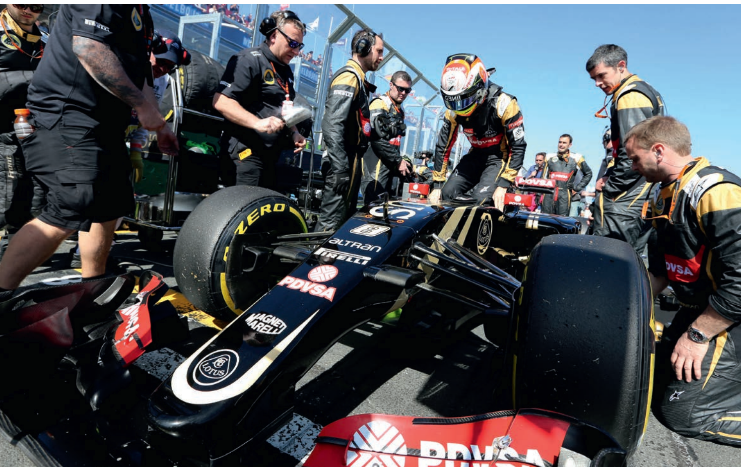
Another consequence of the new nose regulations is that packaging the front suspension has become a much tougher job
